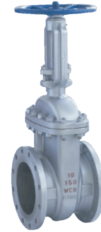
Rising stem Gate Valve (ANSI CLASS150/300/600~900/1500)
